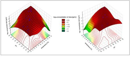
**Figure 4.** A 3D surface plots of relationships between concentration of potentially infectious RoV and AdV viral particles and physical parametres of water samples. The graph is a 3D projection of log10 concentration of viruses, temperature and pH of the samples. The blue dots represent values on which basis the surface were plottes
